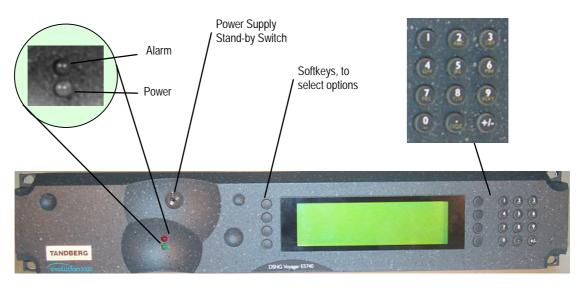
Figure 1.9: 2U Encoder Front Panel Indicators
